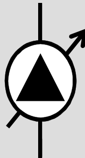
Hydropack 1 pompa inverter
